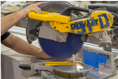
Cut trim & miter corners
