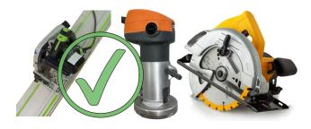
2) Inside corner cuts must be made with ½" diameter router bit.
